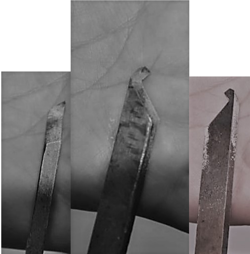
Recess tool side, bottom, top
