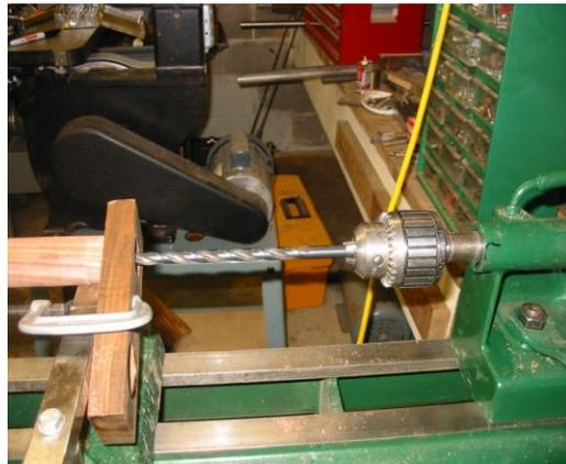
JB Weld both inserts into the blank, taking care to keep the epoxy clear of the backend of the tool insert if the tool needs to slide down into the handle. Allow to dry.
