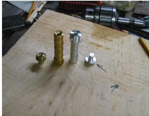
The rear insert is not required but allows you to return or refinish the tool between centers. This insert is made of 3/4 inch round stock which has the internal part turned down to 3/8 inch and the external part left full sized (3/4 ") and finished as you desire. It should be center drilled to allow turning between centers.
